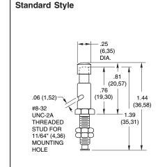
Red/Black cap Part No. 29-100 No cap Part No. 29-110 No cap, high temp. Part No. 29-125
