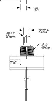
UNLESS OTHERWISE SPECIFIED, DIMENSION TOLERANCES ARE AS FOLLOWS: LINEAR .010 (.25), DIAMETERS .010 (.025), ANGULAR  $5^{\circ}$
