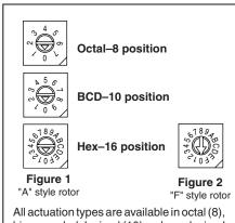
hinary coded decimal (10), or hexadecimal (16) codes; with either standard or complement output. Standard code outputs have natural color rotors; complements in a contrasting color.
