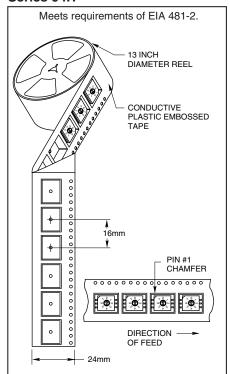
Each reel contains the following number of switches with a 15.35 inch (390 mm) minimum leader and a 6.30 inch (160 mm) minimum trailer.
