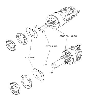
The adjustable stop Series 71 rotary switches allow you to change the number of positions per pole. Simply remove and relocate stop pins in the holes in the front of the switch. The pins are held in place by a self adhesive sticker which fits over the front plate.
