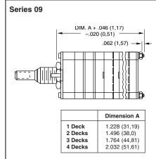
SOLDER DIM. A LUGS PC TERMINALS
